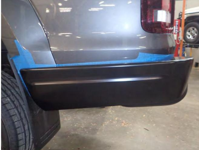
81. With the assistance of other people or a lifting device, position the wings next to the rear side vehicle panels. Take care not to damage the vehicle when positioning the wings.
