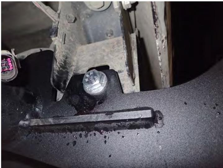
39. When fitting bar to the vehicle on MY 11-16 vehicles, fit M12 Bolt and washer and M12 Nut plate in to chassis rail
