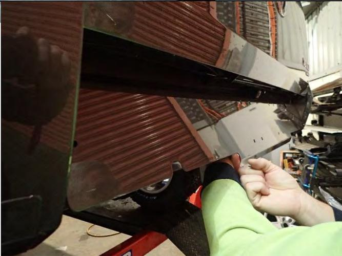
43. Install Beaver Panel. Insert 4 x M6X20 bolt and washer through beaver panel and position spacer as shown
