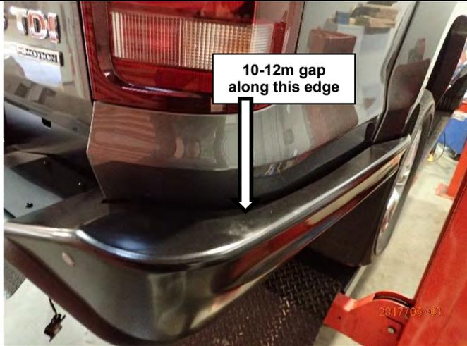
85. Position each wing so there is an even 10-12 mm gap to the side vehicle panels.
