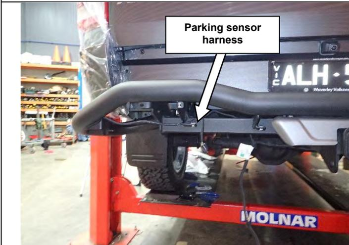
55. Route the trailer plug loom and parking sensor loom through the RSTB and attach to the appropriate connector on the RSTB wiring harness or vehicle loom as shown.
