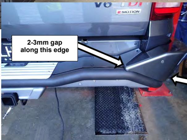
87. Position each wing so they sit evenly on the step plate and there is an even gap to the tube as shown.
