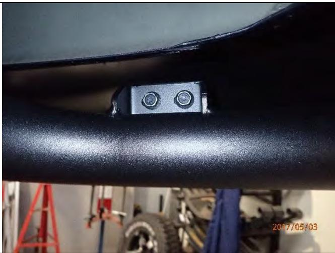
84. Fix the middle bracket of each wing to the RSTB tube using 2 X M8x1.25x20 hex head flanged bolts and the wing double nut plate already fitted. Leave bolts finger tight at this stage.
