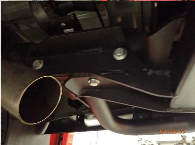
52. Fix the RSTB to the threaded holes in each chassis rail using 1 M12 x 1.25x40 (fine pitch) hex head bolt, 1 M14 x 110 bolt and nut. Leave finger tight at this stage.
