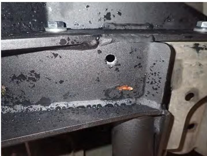
40. With the rear bar fitted. Mark and drill 1 x  $\text{Ø}13\text{mm}$  hole on the bottom face of both chassis rails.
