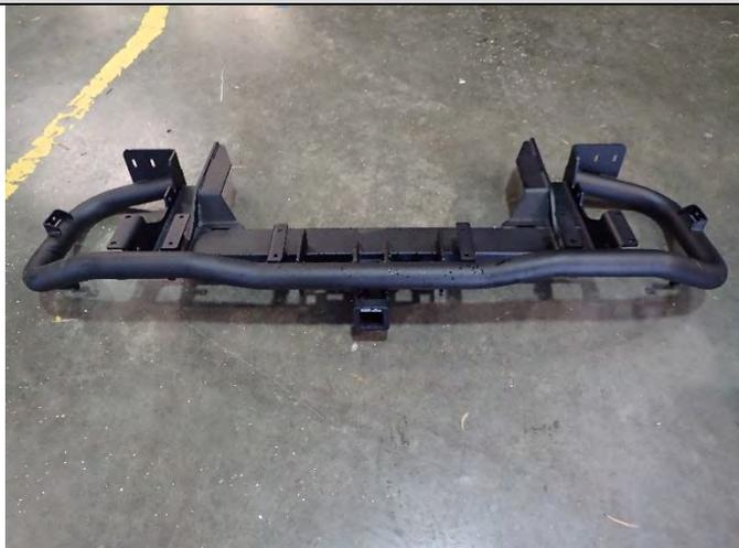
28. Place the RSTB on a flat surface that will not damage its coating as shown.
