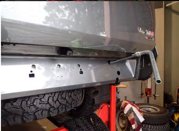
4. Remove the spare wheel from beneath the tub using the wheel nut wrench and jack handle pieces supplied with the vehicle.
