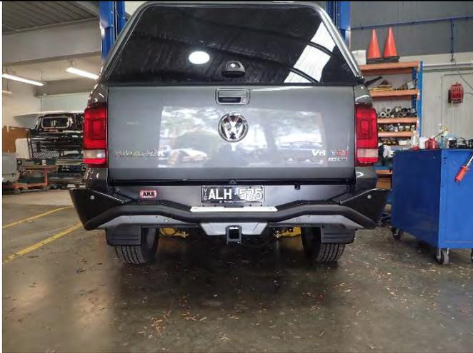
94. Reattach the spare wheel beneath the vehicle. Store tow tongue, pull pin and R-clip in a safe and secure location when not in use.
