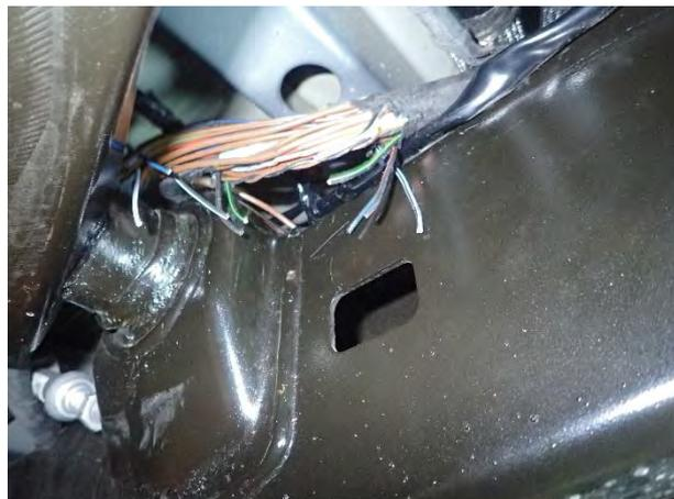
**Note: Prior to cutting the exposed wires, please ensure and re-check (with a test light or multimeter) that the correct wires have been identified as per their corresponding function, as there are multiple wires of the same colour in the vehicle loom.**
