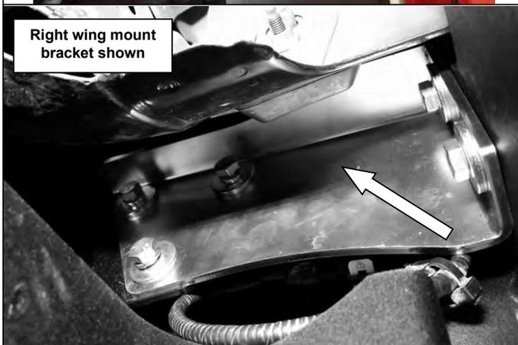
83. Fix the wing mount bracket of each wing to the RSTB using 2 X M8x1.25x25 hex head bolts, 4 M8 flat washers and 2 X M8 nuts. Do not fully tighten at this stage.
