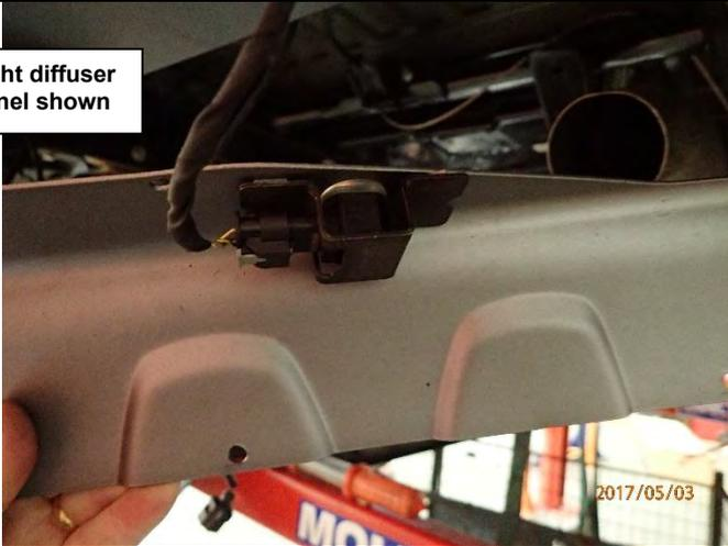
89. Attach the rear parking sensor with 3M double sided tape to the diffuser panel, ensure the sensor is centre in the hole.
