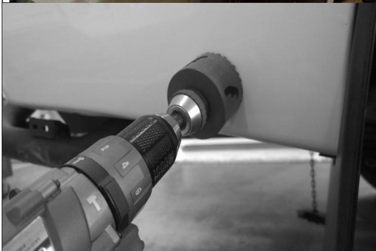
72. Using a Ø70mm hole saw, drill through the rear side panel using the mark from the previous step as the centre point of the hole.
