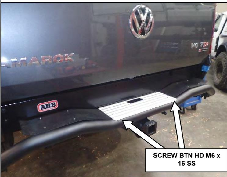
68. Attach the step plate extrusion to the RSTB using 4 x stainless steel M6x1.0x16 button head screws.
