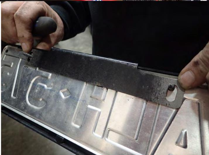
48. Prior to fitting licence plate, place 'Light Deflecting Bracket' behind licence plate as shown. Then screw the licence plate and bracket to Beaver panel.
