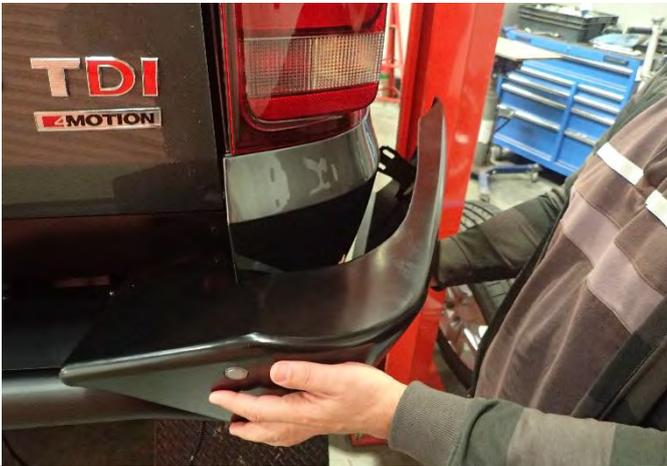
80. With the assistance of other people fit the rear parking sensor and bracket to the wing and fit the wing to the centre mount using 2 X M8x1.25x25 hex head bolts and nuts.
