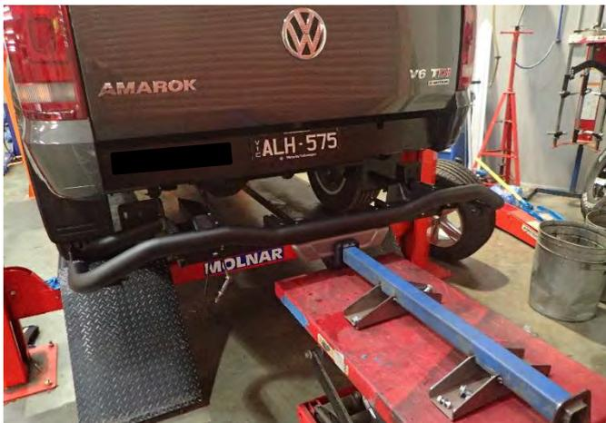
51. With the assistance of other people or a lifting device, lift the RSTB up beneath the chassis rails aligning the threaded holes in the side of the chassis with those in the vertical surfaces of the RSTB.
