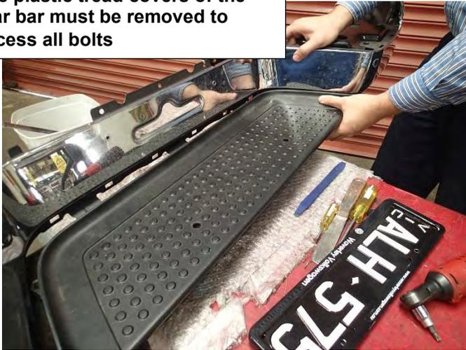
5. Once the bumper assembly has been removed from the vehicle, the bumper assembly must be disassembled to remove the rear parking sensors and harness.
