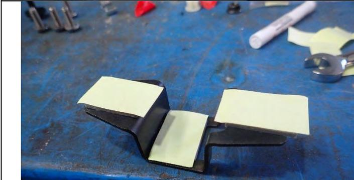
**Note:** Ensure the parking sensor bracket is clean and free of residual tape and foreign matter.
