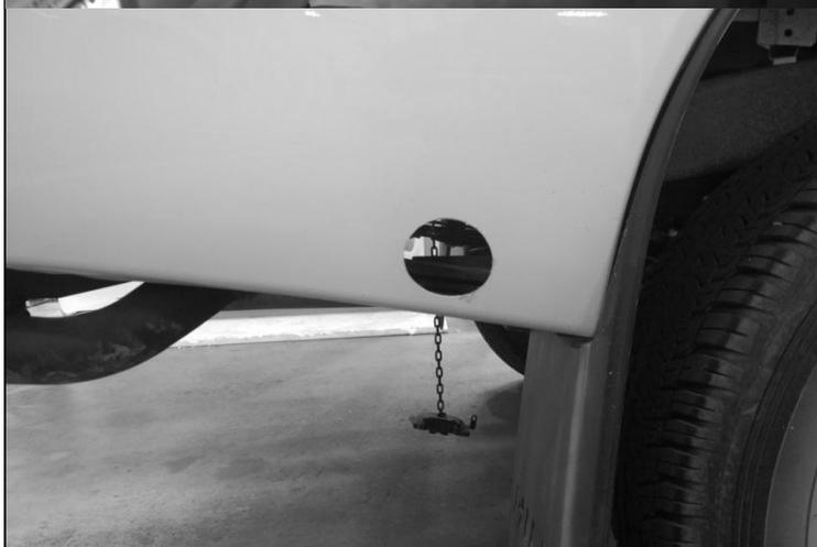
74. De-bur each hole to remove sharp edges.
