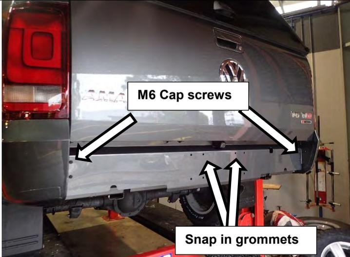
46. Fit 4 x M6 cap head screws and washers to fix beaver panel to beaver panel bracket
