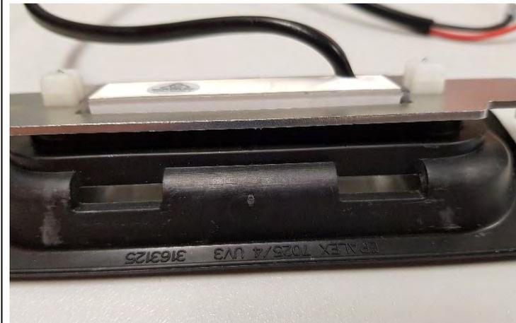
60. **Remove the foam ring from the LED lamp and discard.**
